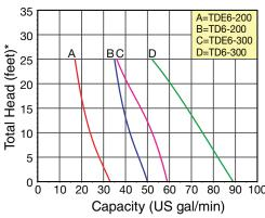
(\*) Convert to psi, divide by 2.31 Liquid - Water specifc gravity 1.0
