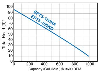
\* Convert to PSI, divide by 2.31 • Liquid-Water specific gravity 1.0
