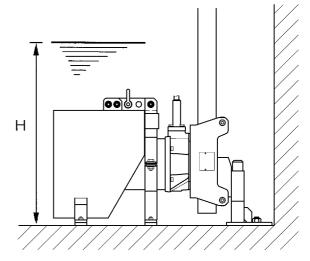
Even when using the operating water level shown above, swirls may emerge on the water surface depending on the pit shape or the installation position. In such a case, raise the water level.
