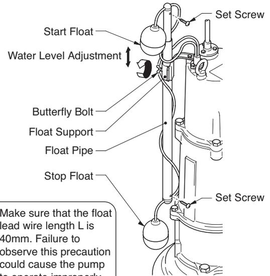
To change the operating water level on an automatic alternating model, perform the setting by referring to the diagram on the right.
