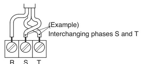
**Note:** This method cannot be used if the starting panel is equipped with a reverse-phase detector such as a 3E relay. If this is the case, contact the manufacturer of the starting panel, the dealer where the pump was purchased, or the Tsurumi sales office in your area.
