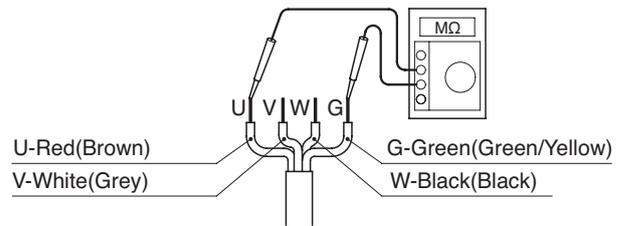
Insulation resistance reference value = 20M  $\Omega$  minimum
