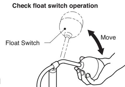
**Note:** It takes approximately 1 second for the pump to start after the float is moved. Allow the pump to operate a minimum of 2 seconds for each trial operation. The trial operation must be completed within 1 minute.
