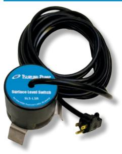
The Surface Level Switch with Lift Bracket is used to automate a utility/ floor sucking pump. Set the Surface Level Switch on the floor and plug the power cord from the pump into the piggyback plug on the switch. Plug the piggyback plug into a standard 120 VAC wall outlet (the unit will also work on GFI outlets).
