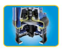
**NEW** Tsurumi Agitator Pump **KTD Series** is a cast iron made, heavy-duty slurry pump employing the KTZ Series as the base. An agitator is provided to assist smooth suction of the pumping fluid. The side-flow, top-discharge design keeps the motor cooling even if the pump is operated continuously with its motor exposed in air, and it makes the pump easier to place in a confined space.
