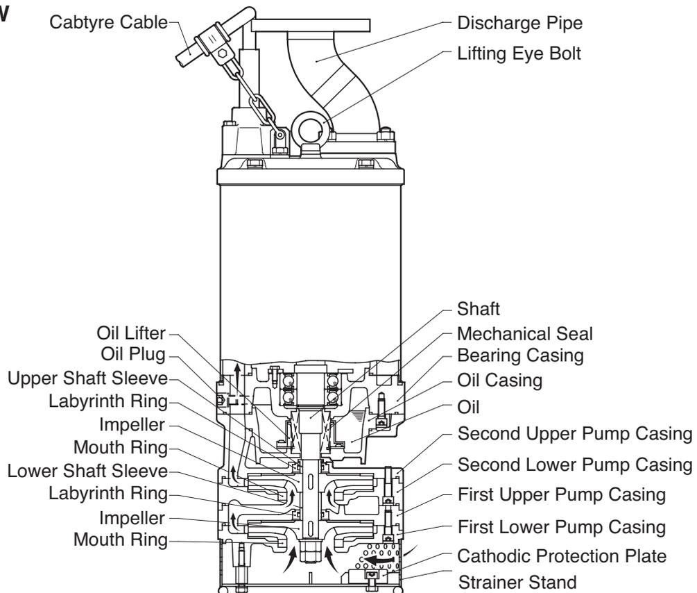
**Note:** *The above diagram is typical of the LH-W Series, but some models may vary slightly in appearance or internal structure.*
