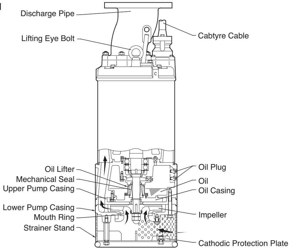
**Note:** *The above diagram is typical of the LH Series, but some models may vary slightly in appearance or internal structure.*
