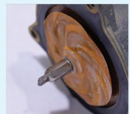
After 200 hours operating in a 15% silica sand slurry, the urethane impeller maintained its original profile while the cast iron impeller experienced severe erosion, resulting in substantial performance loss.
