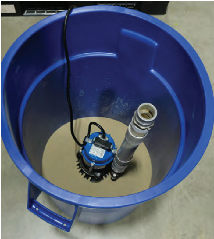
A large test tank containing a silica sand slurry was used to simulate severe abrasive pumping conditions during the 200-hour endurance test.
