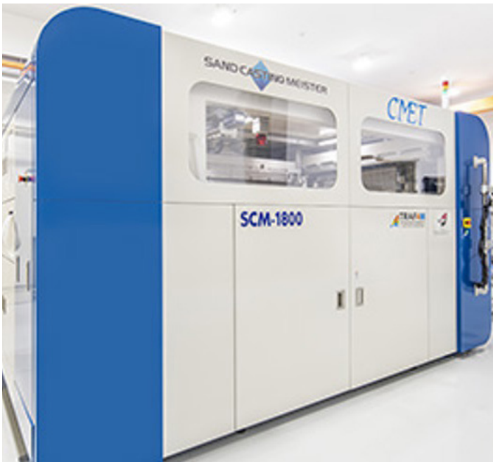
Artificial Sand 3D Printer at the Molding Research Building
