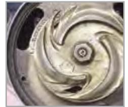
Competitor Impeller is effectively worn out.
