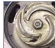
Competitor Impeller is effectively worn out.
