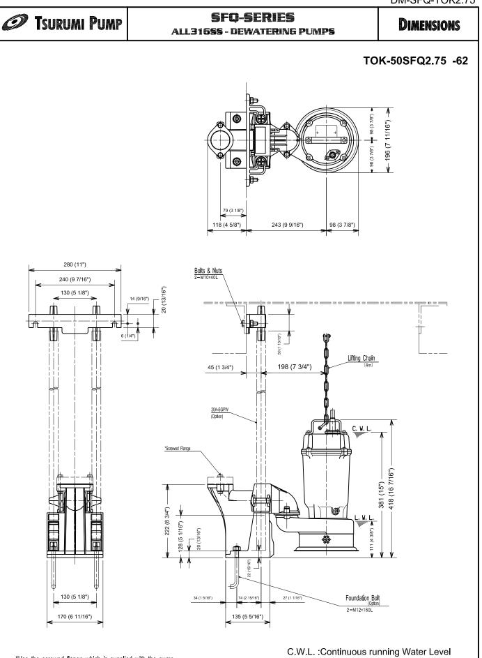
\*Use the screwed flange which is supplied with the pump.
