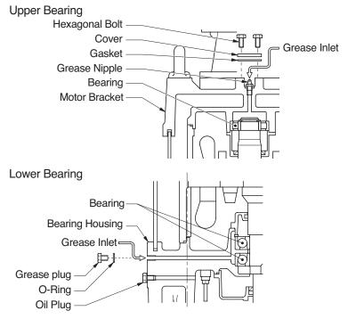
**Note:** Greasing generally is good for around 3,000 hours of use, but this can vary depending on the use conditions.
