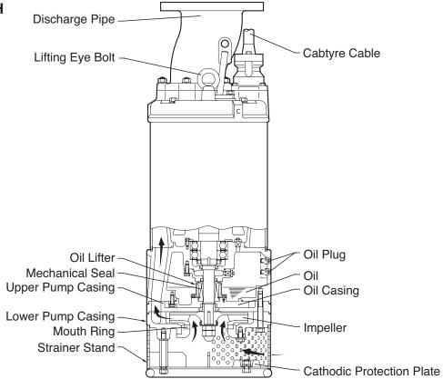
Note: The above diagram is typical of the LH Series, but some nodels may vary slightly in appearance or internal structure.
