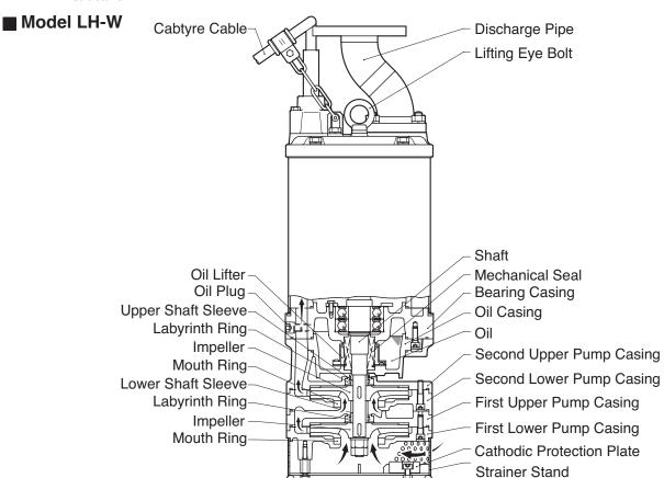
**Note:** The above diagram is typical of the LH-W Series, but some nodels may vary slightly in appearance or internal structure.
